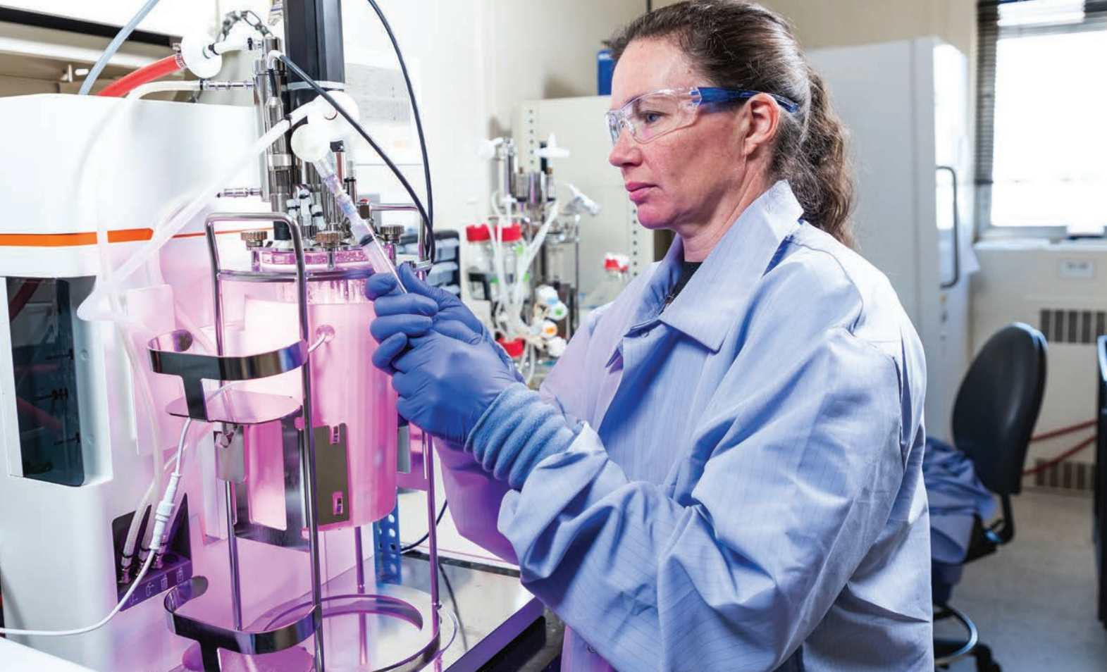
■ Sara Pacheco works with a bioreactor, the system responsible for using algae to fix carbon into molecules that are then modified by the chemistry team to produce sustainable aviation fuel.
