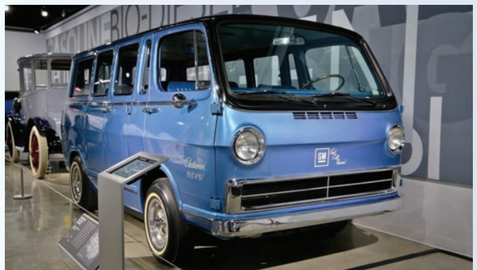
■ General Motors' Electrovan was the first fuel cell electric automobile. The vehicle's limitations were such that only one Electrovan was ever produced. Photo: Speedhunters/Mike Garrett
